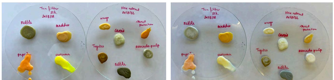
Left picture shows samples of colored soy wax before UV exposure. Right picture shows the effect of 1 month UV exposure. The left plate contains 'infused' samples of soy wax, while the right plate holds 'hexane extract' samples.
