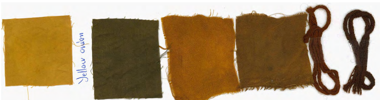
Textile pieces dyed with yellow onion extract. From left to right: cotton alum – cotton iron – silk alum – silk iron – wool alum – wool iron.
